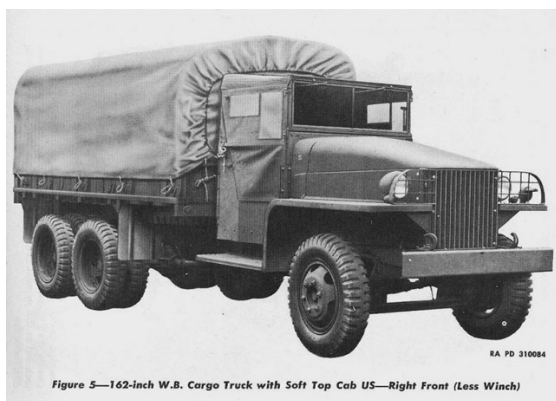
Figure 5—162-inch W.B. Cargo Truck with Soft Top Cab US—Right Front (Less Winch)
